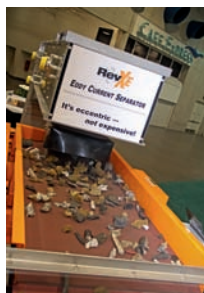
Eriez' RevX-E Eddy Current Separator featuring an eccentric magnetic rotor to allow a single point of separation.
