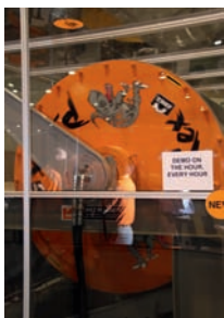
Eriez' new P-Rex, a permanent rare earth 'Xtreme' drum magnet for automotive shredder residue processing.
